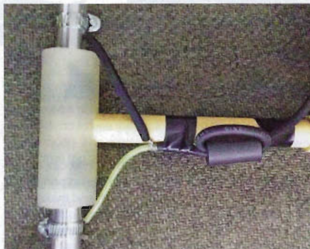
Figure 4 — Match by spreading the coax leads where they connect to the aluminum elements. In this version, K4ERO used a single, large toroid with two turns of coax.
