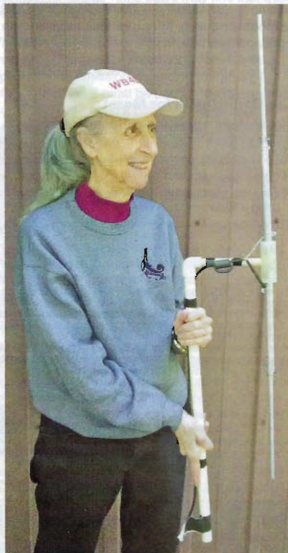
Figure 1 — Ruth Stanley, WB4LUA, shows the utility antenna setup for 2-meter FM with vertical polarization.
