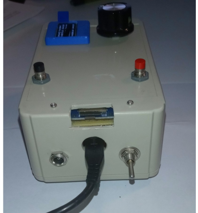
The two ends. Left: the four channel outputs. Right: power inlet, toggle switch, and the microSD slot.
