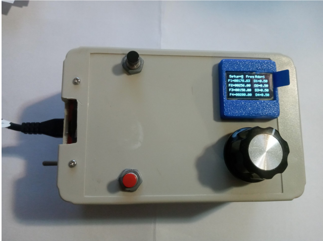
The Generator in its enclosure, with the 3D-printed display frame.
